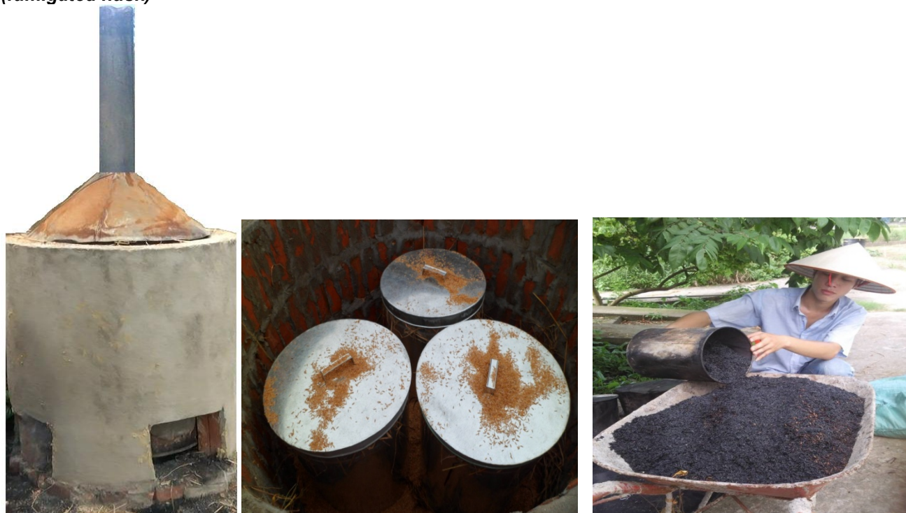
Figure 12: Production of Bio-char from inearobic charring of rice husk through indirect pyrolysis (fumigated husk)
