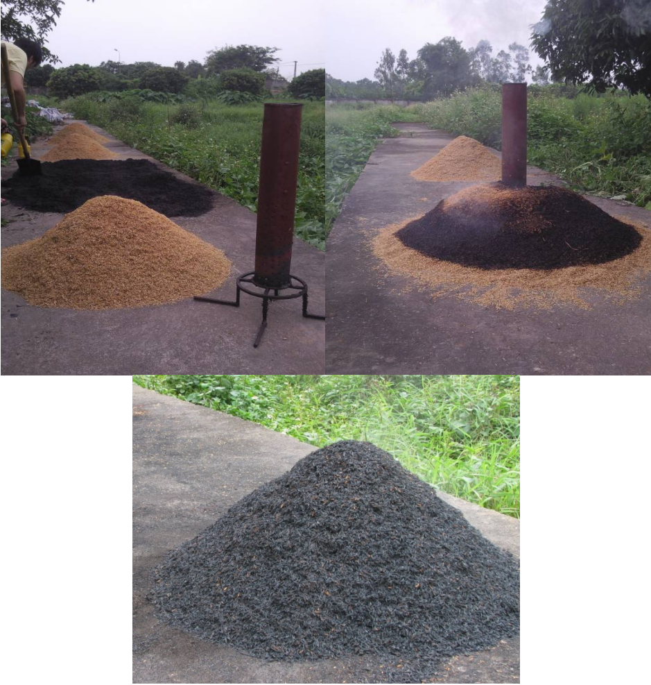
Figure 11: Rice husk burning to produce biochar through chimney
