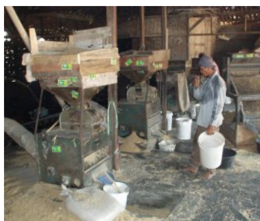
Picture 4: Single pass, two stage rice mill (picture from rice knowledge bank, 2009)
