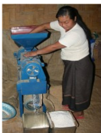
Picture 3: Single pass, single stage rice mill for home use (Picture from rice knowledge bank, 2009)
