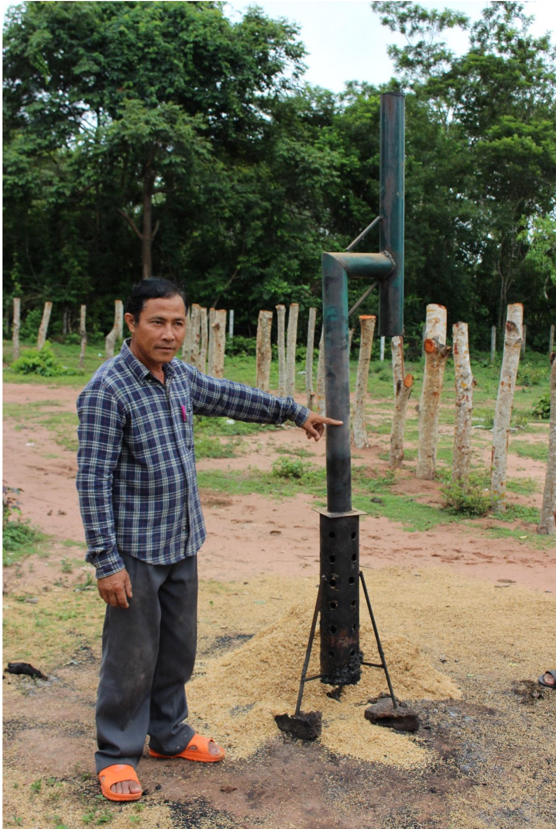
Simple biochar production equipment used at the communal facility at village Pai in Champone district.
