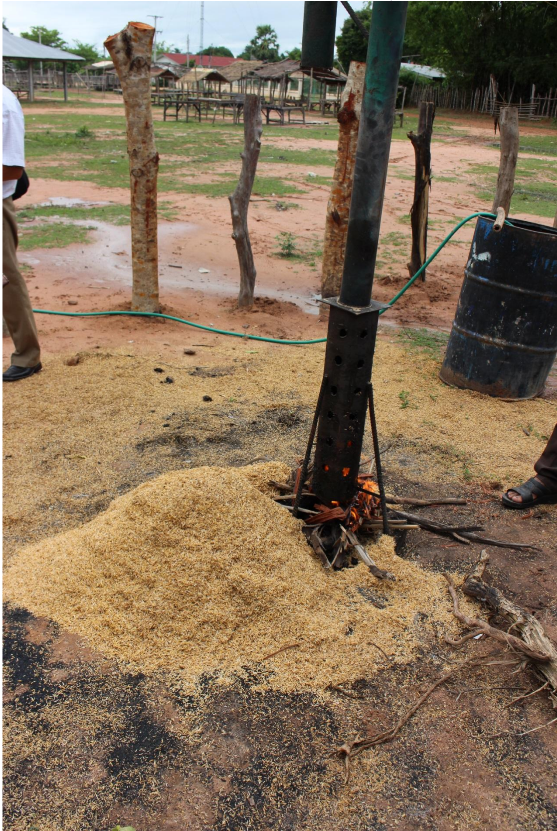
A demonstration of biochar production from rice husk at the communal facility at village Pai in Champhone district.
