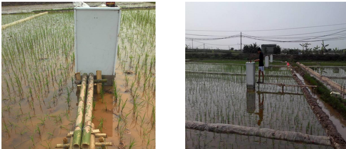
Figure 5: Chamber Method for Sampling and Measuring Methane and Nitrous Oxide Emissions
