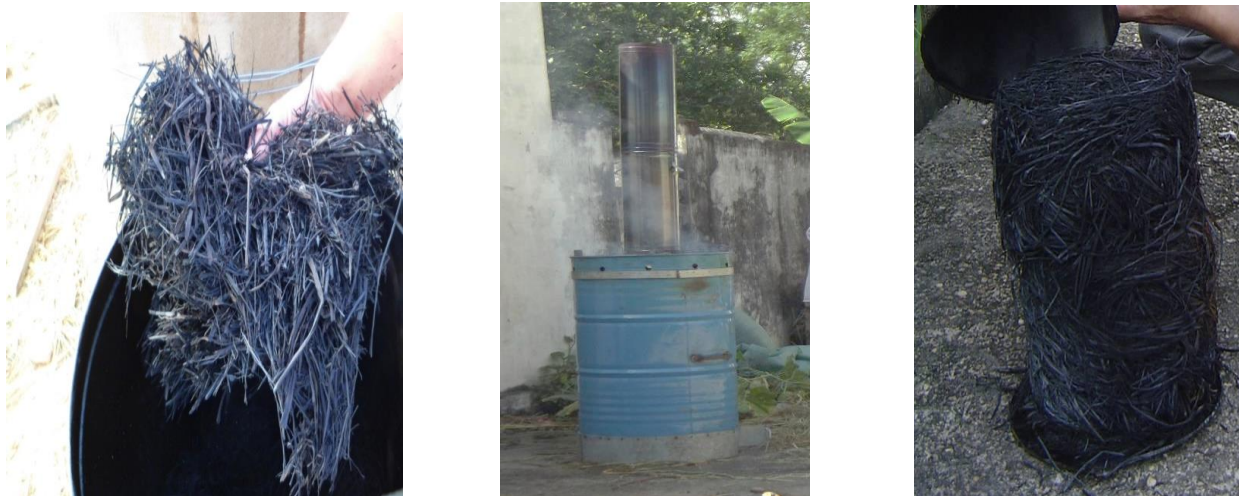
Figure 3: Producing Biochar from Rice Straw, Using a Kiln
